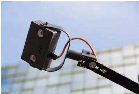
SCOOT (Split Cycle Offset Optimisation Technique) monitoring equipment
