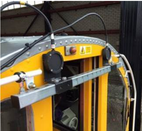
Battery loco testing with Thales ATC radio system at Old Dalby
